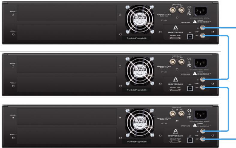
Utilize an Avid Sync HD by connecting its Loop SyncHD Option Card Loop Sync connections in the same way:
