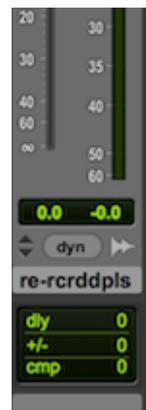
Delay compensation values are now displayed at the bottom of each Mixer channel.
