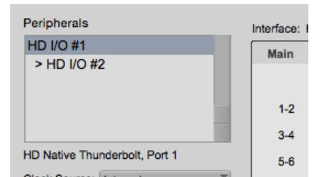
Each HD I/O transmits and receives 16 channels of audio. These 16 channels of audio are detected regardless if it's a 16x16, 8x8, or 2x6 module card.
