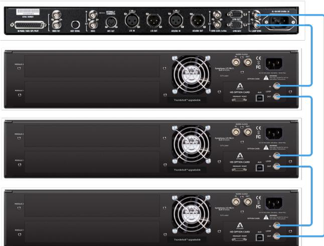
Utilize an external master clock into your system by connecting to the regular Word Clock, then use Loop Sync for the rest of your HD hardware:
