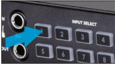
1. Press and hold the desired Input Select button for at least **1 second**.
