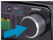
3. Press the Output knob to toggle the monitor output mute on and off.
