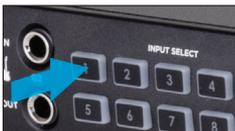
4. Press and hold the Input Select button for at least **1 second** to return to the Input level meter screen.
