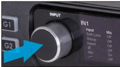
3. Press the Input knob to change the input source.
