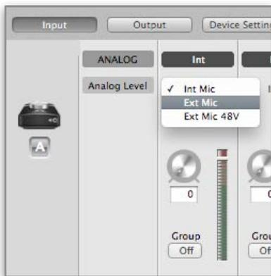
Select the Analog Level setting that corresponds to the microphone source you'd like to record. For example, if you have a microphone connected to the XLR connection on the breakout cable, select "Ext Mic" from the Analog Level menu on channel 1. If you would like to utilize ONE's built-in microphone, select "Int Mic". By default, the 1/4" instrument input is the selected source for Channel 2.
