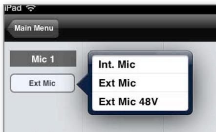
Select the Analog Level setting that corresponds to the input source you'd like to record. For example, if you have a microphone connected to the XLR connection on the breakout cable, select "Ext Mic" from the Analog Level menu on channel 1. If you would like to utilize ONE's built-in microphone, select "Int Mic". By default, the 1/4" instrument input is the selected source for Channel 2.
