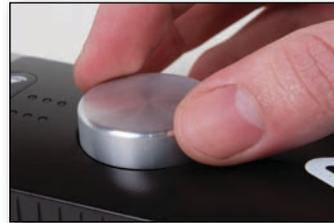
The controller knob operates in parallel with any software output controls.
