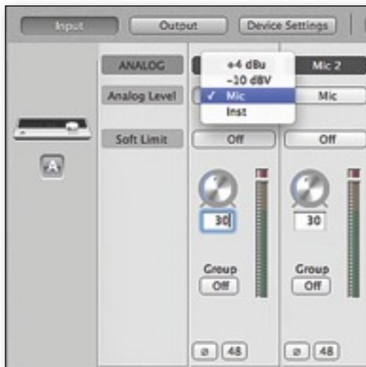
Select the Analog Level setting that corresponds to the device you have connected to Quartet's input(s). For example, if you have an XLR microphone connected to input 1, select "Mic" from the Analog Level menu on channel 1. If you have a 1/4" instrument connected to the input, then select "Inst"
