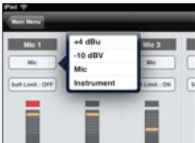
Select the Analog Level setting that corresponds to the device you have connected to Quartet's input(s). For example, if you have an XLR microphone connected to input 1, select "Mic" from the Analog Level menu on channel 1.
