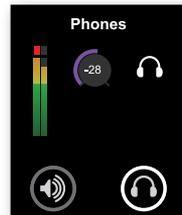
The controller knob operates in parallel with Maestro's headphone control.
