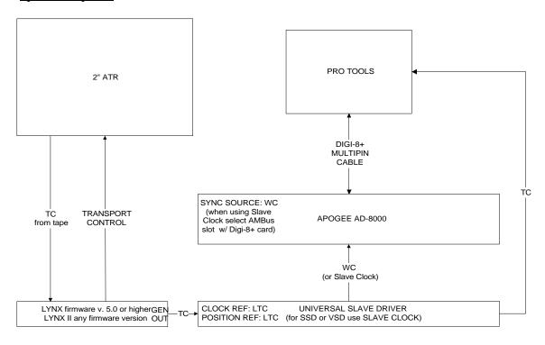
The idea is to have the Lynx control the 2" transport. The time code from tape is fed into the Lynx. The TC is then regenerated (referenced to the Lynx's internal crystal) and output to the USD. The USD is consequently always receiving fresh TC referenced to a stable crystal source (the same source that is controlling the ATR transport). Your digital audio won't suffer from the inconsistency in speed (wow and flutter) of a "wild" analog tape recorder.
