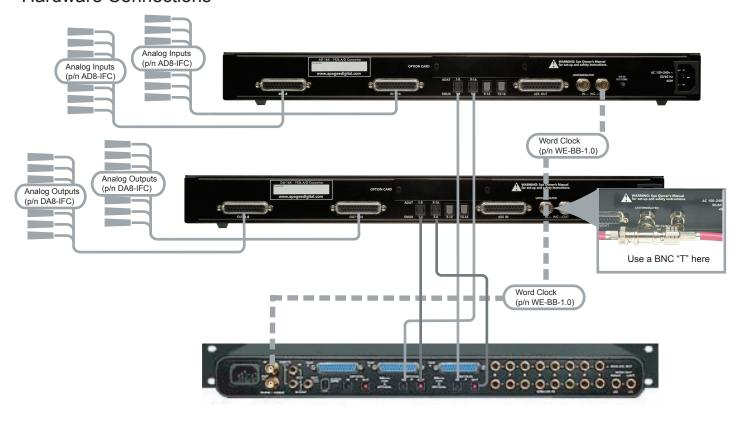
Connect AD-16X WC Out to a BNC "T" connector installed on DA-16 WC In. Connect the other side of the BNC "T" connector to the MOTU 2408 WC In; do not terminate this input. Alternatively, use an Apogee Big Ben as a Master Clock and connect each device to it's own Big Ben WC Output.
