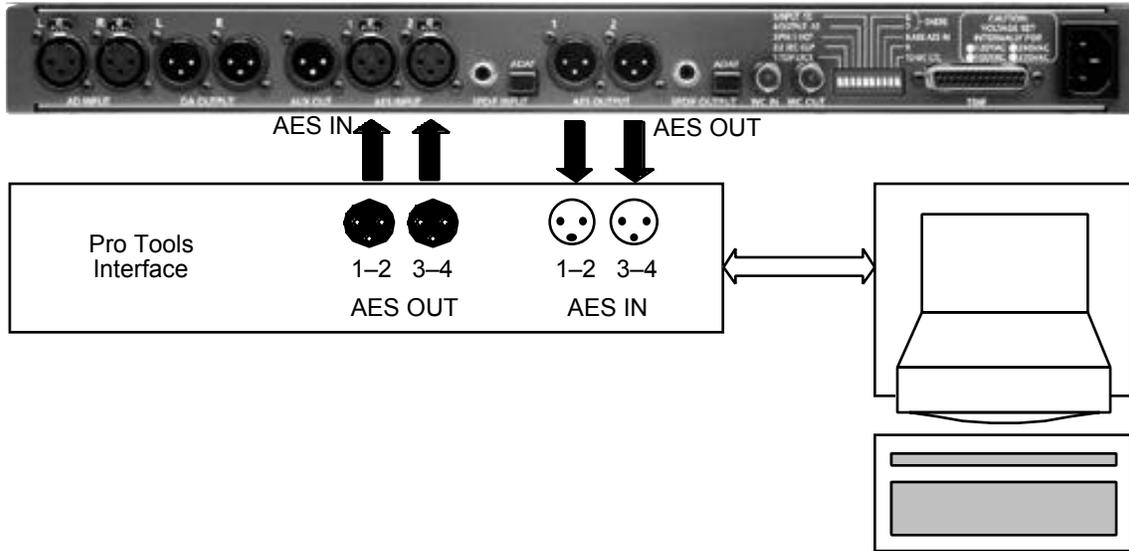
*Connecting the PSX-100 to your Pro Tools interface: Simply connect the two AES outputs of the PSX-100 to the first two AES inputs on your interface; and connect the PSX-100's AES outputs to receive signals from the first two outputs of the Pro Tools unit. That's it!*
