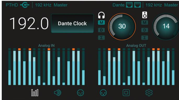
For the purposes of getting started quickly, it's recommended to set the Symphony I/O clock source to Dante Clock from the front panel OLED. Tap the Meter icon, then tap the clock source button, then choose Dante Clock in the scroll down list, then tap OK. When Symphony I/O is set to Dante AIM, routing between the I/O modules and the Dante network is fixed in a “one-to-one” setting as shown.
