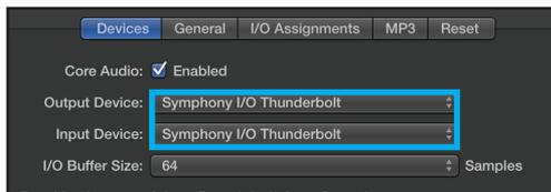
3. Start by setting the I/O Buffer Size to “64 Samples”. Adjust the setting based on your computer’s performance.
