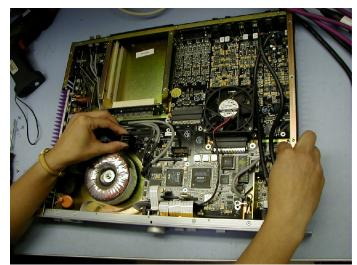
Make sure that both the DAC and analog board connector (by the fan) are lined up with the respective connectors of the digital board and pull boards together until connections are snug. Reistall all screws and top.
