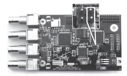
Please note that when an X-Video card is installed in a Big Ben, Big Ben's chassis-mounted Video/Word Clock BNC input will *only* accept word clock signals; video reference input signals should be connected to the X-Video **IN** BNC connector.
